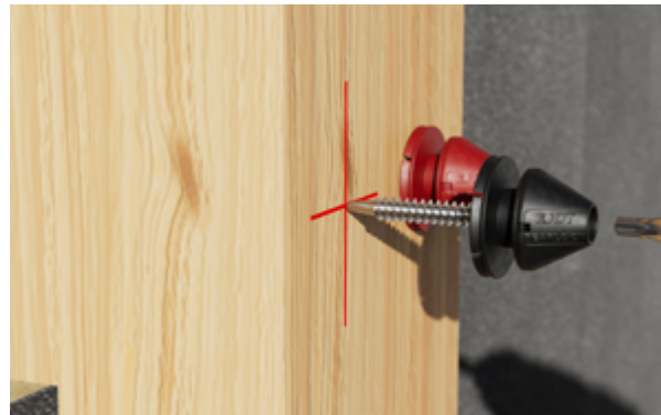
Position the PEARLOCK® system on the timber substructure and fasten it with the LT-XT screw using the extended TX25x70 bit.
